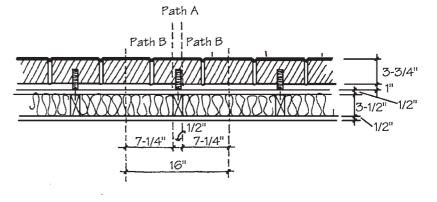
Stud spacing = 16.00 in. o.c., or 1.33 ft o.c. Height of the section = 12.00 in. or 1.00 ft Total area,  $A_t = 1.33 \times 1.00 = 1.33$  sq ft Width of Path A = 1.50 in. or 0.125 ft Area of Path A,  $A_A = 0.125 \times 1.00 = 0.125$  sq ft Width of Path B = 16.00 - 1.50 = 14.50 in. or 1.208 ft Area of Path B,  $A_B = 1.208 \times 1.000 = 1.208$  sq ft
